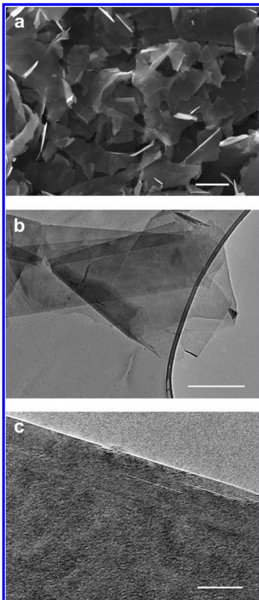
**Figure 1.** Micrographs of graphite flakes. (a) SEM image of graphite flakes obtained by the  $\text{H}_2\text{SO}_4$  intercalation, microwave expansion, and ultrasonic exfoliation of natural graphite; scale bar: 2  $\mu\text{m}$ . (b) Typical TEM image of a graphite flake; scale bar: 500 nm. (c) HRTEM image of a graphite flake; scale bar: 10 nm.
