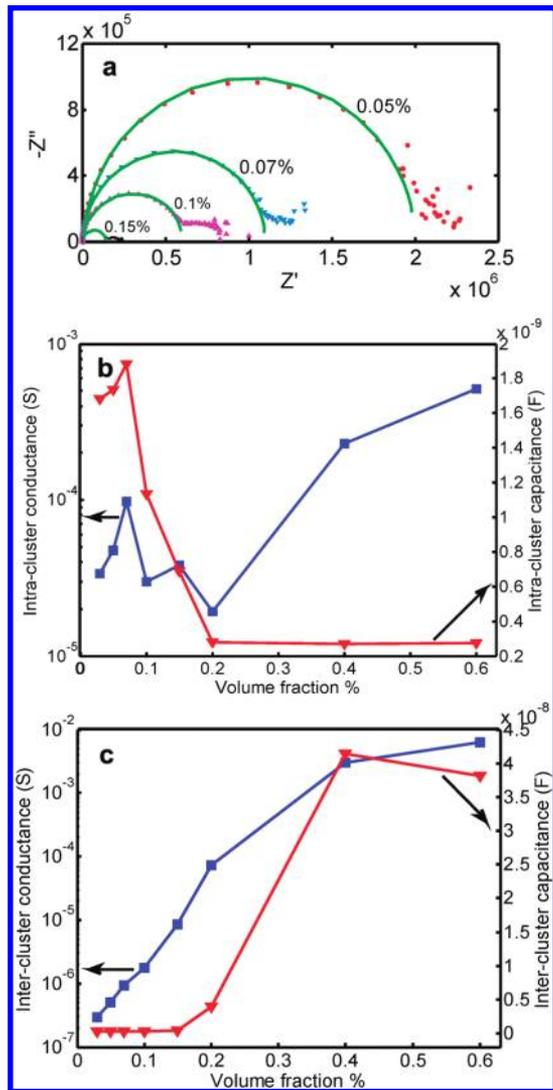
**Figure 4.** Electrical characteristics of EG/graphite suspensions corresponding to the red curve in Figure 2(c) (25 min ultrasonic time). (a) Nyquist plots of AC impedance of EG/graphite suspensions at different volume loadings, and (b) intra- and (c) intercluster conductance and capacitance as a function of graphite volume fraction.
