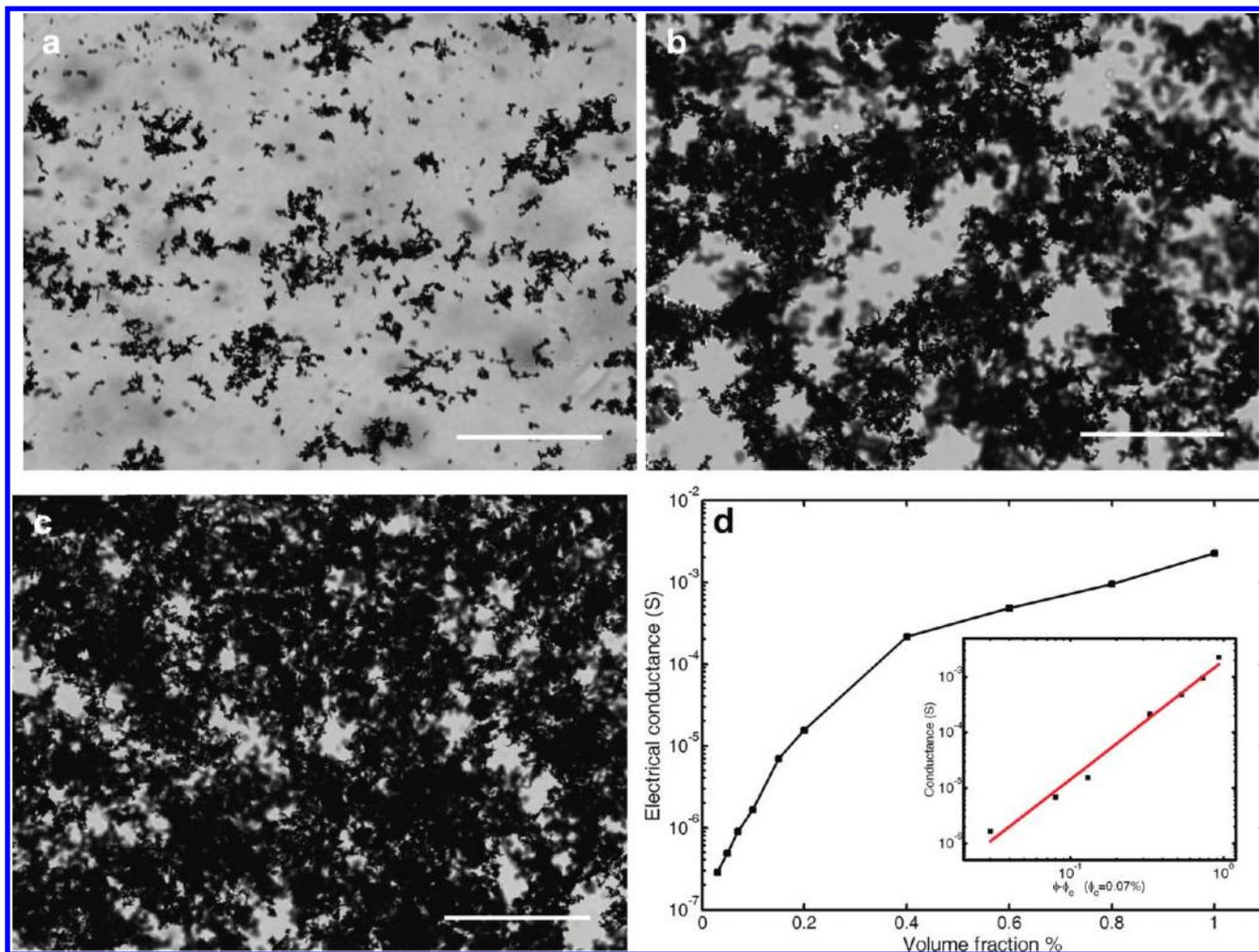
**Figure 3.** Optical micrographs of the microstructures of graphite/EG suspensions at three volume fractions: 0.03% (a), 0.1% (b), and 0.2% (c). Scale bars in a–c are all corresponding to 200  $\mu\text{m}$ . (d) Electrical conductivity shows a percolation behavior at 0.07%.
