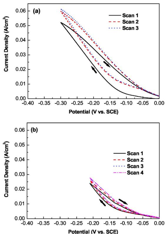
**Figure 6.** (Color online) Variation of voltammetric switching potential [(a)  $-0.3$  V, (b)  $-0.21$  V] in the SPS-PEG-Cl system. The sweep rate was  $1$  mV/s.
