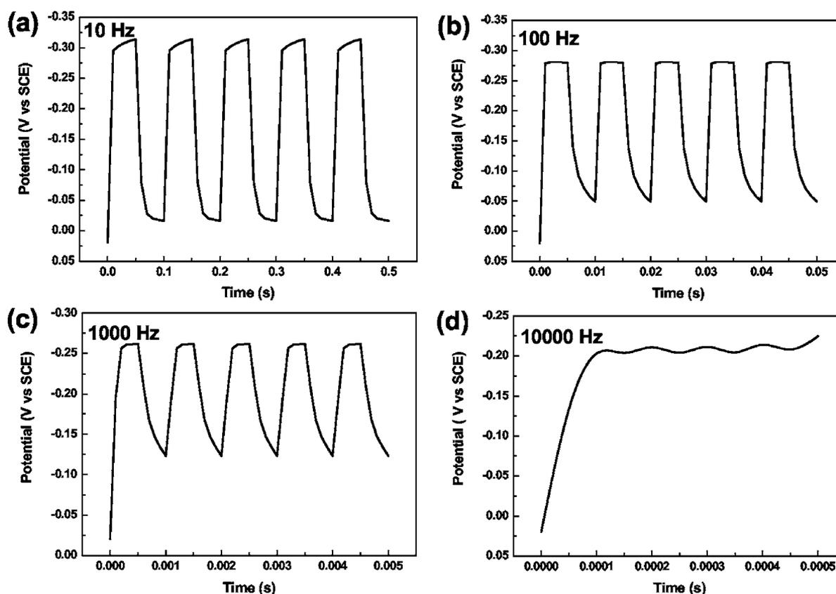
Figure 5. Potential responses with time at various pulse frequencies in the bath with additives, SPS + PEG +  $\text{Cl}^-$ . The applied average current density is  $10 \text{ mA/cm}^2$ .
