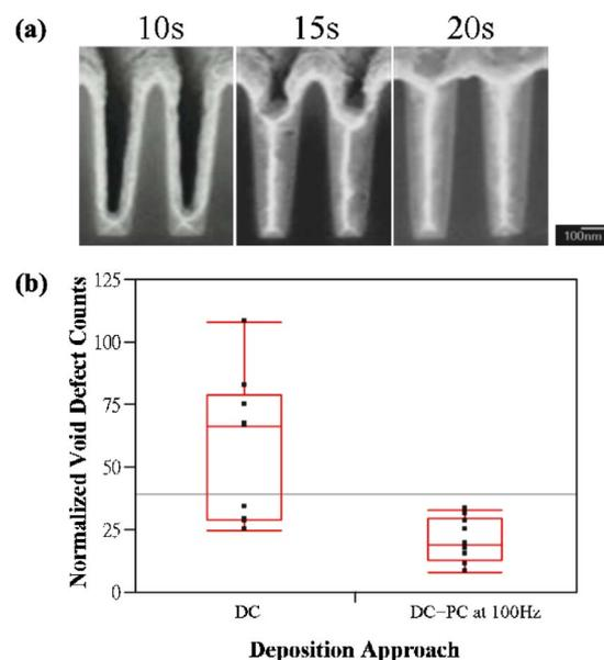
**Figure 9.** (Color online) (a) SEM images of filling experiments in different deposition time. (b) Box plot comparison between only dc and dc + PC at 100 Hz pulse frequency deposition approach for the formation of void defects on pattern wafers.
