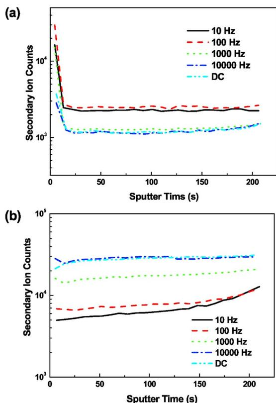
**Figure 8.** (Color online) Secondary ion counts for (a) sulfur and (b) chloride in copper deposits at various pulse frequencies in the bath with additives, SPS + PEG + Cl<sup>-</sup>, are plotted against the sputtering time. The applied average current density is 10 mA/cm<sup>2</sup>.
