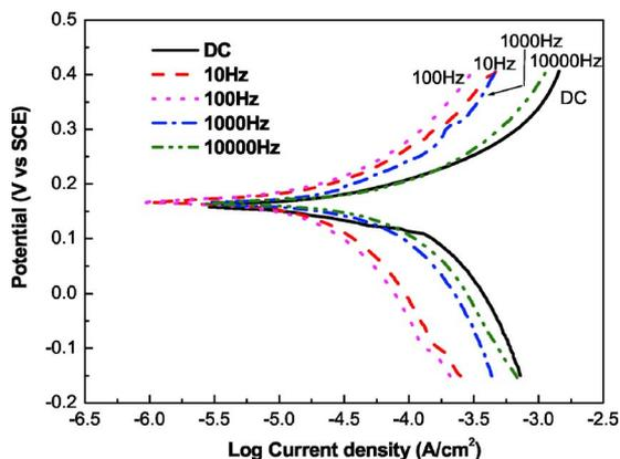
Figure 3. (Color online) Potentiodynamic polarization of copper deposits plated at various pulse frequencies after annealing immersed in commercial polishing slurry.
