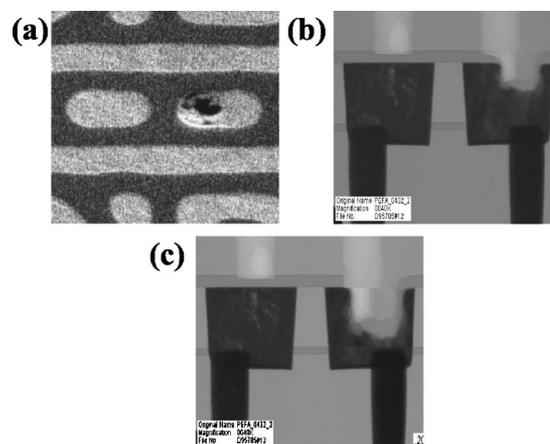
**Figure 1.** Images of void defect to show the influence of void defect on fabrication of multilayer interconnect. (a) Top-view of void defect. (b) Cross-sectional image of void defect. (c) Cross-sectional image of void defect after photolithograph and etching processes.
