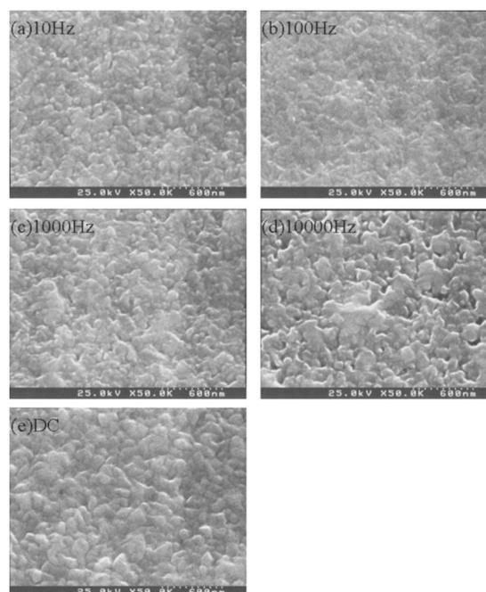
**Figure 7.** Surface morphology of copper deposit with PC plating at various frequencies as well as with dc at  $10$  mA/cm<sup>2</sup> in the bath with additives, SPS + PEG +  $\text{Cl}^-$ .
