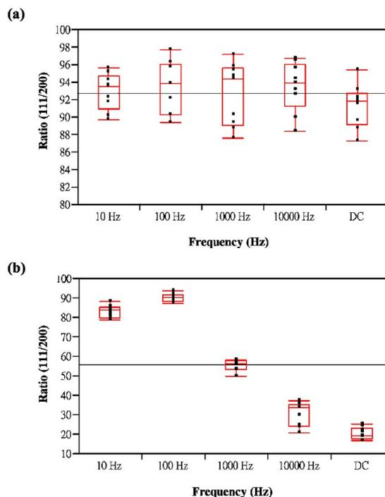
Figure 2. (Color online) Effects of PC frequency on the crystal orientation of copper deposits (a) without and (b) with annealing.
